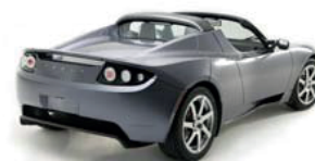
Slika 20.22 Tesla Roadster: 15 kWh na 100 km. www.teslamotors.com.
